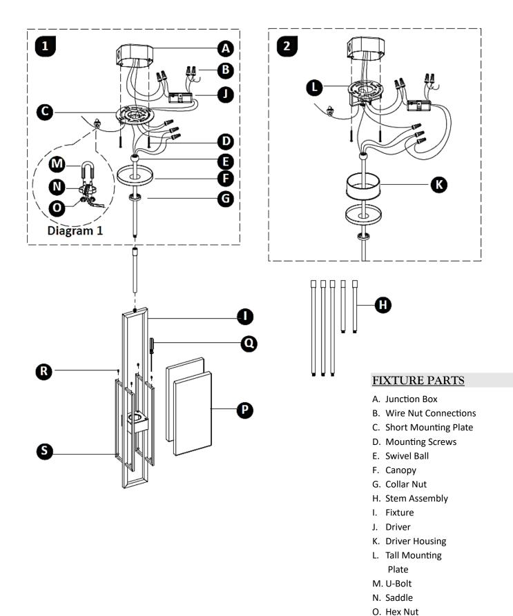
**Please Note:** The tall/short mounting plates and driver housing will not be used for junction box mounted assembly. Keep these parts for future use.
